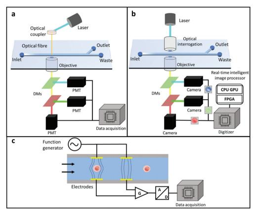
Fig. 3 Schematic of sample detecting system setups in microfluidic flow cytometry. Typical methods are based on (a) optic-based detection, (b) image-based detection, and (c) impedance-based detection.
