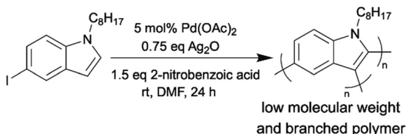
Scheme 10 Room-temperature DARp of 5-iodo-1-octylindole monomer.
