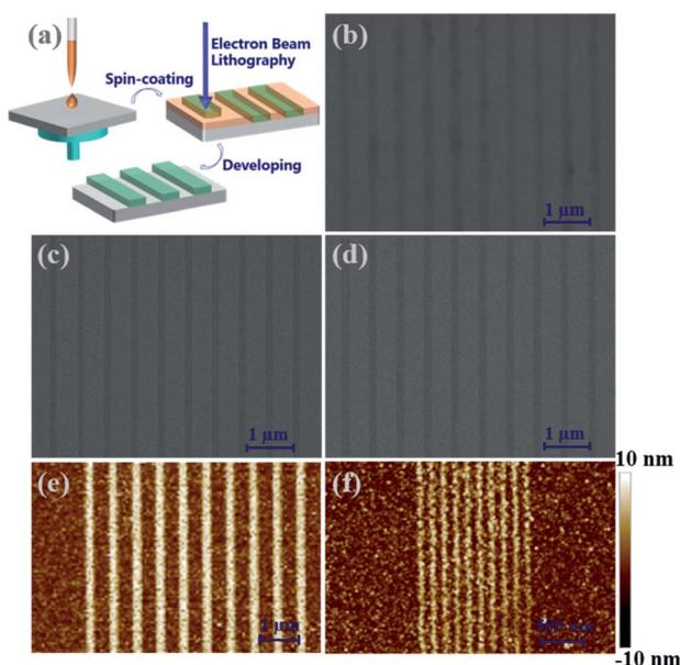
Fig. 4 (a) Schematic illustration of the patterning process of  $\text{In}_{12}$ -oxo clusters. SEM images of patterns with 200 nm lines obtained using electron-beam lithography performed with a dose of 1000  $\mu\text{C cm}^{-2}$  for **InOC-1** (b), **InOC-2** (c) and **InOC-3** (d). AFM images of patterns obtained with a dose of 500  $\mu\text{C cm}^{-2}$  exhibiting feature sizes of 200 nm (e) and 50 nm (f) for **InOC-3**.
