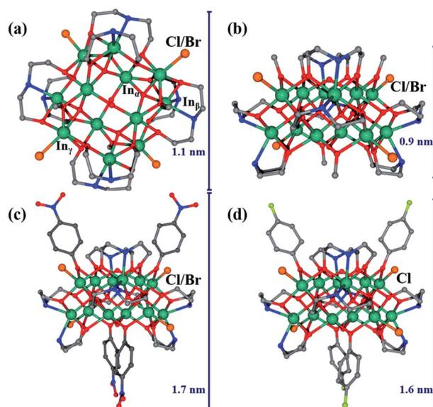
Fig. 1 (a) Molecular structure of **InOC-1** and **InOC-2** in top views. (b) Molecular structure of **InOC-1** and **InOC-2** in side views. (c) Molecular structure of **InOC-3** and **InOC-4** in side views. (d) Molecular structure of **InOC-5** in side views. Atom color code: dark-green, In; red, O; blue, N; gray, C; orange, Cl or Br; lime, F. All H atoms have been omitted for clarity.
