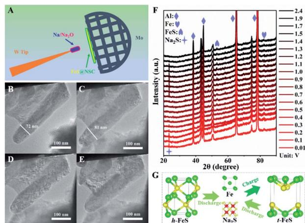
Fig. 5 (A) Schematic illustration of *in situ* TEM experiment during the sodiation process; (B–E) TEM images of FeS@NSC during different sodiation/desodiation processes: (B) initial stage, (C) sodiation, (D) desodiation, and (E) sodiation; (F) *in situ* XRD patterns of the FeS@NSC electrode after the initial discharge; (G) atomic model of the phase change of FeS@NSC during the discharge and charge processes.
