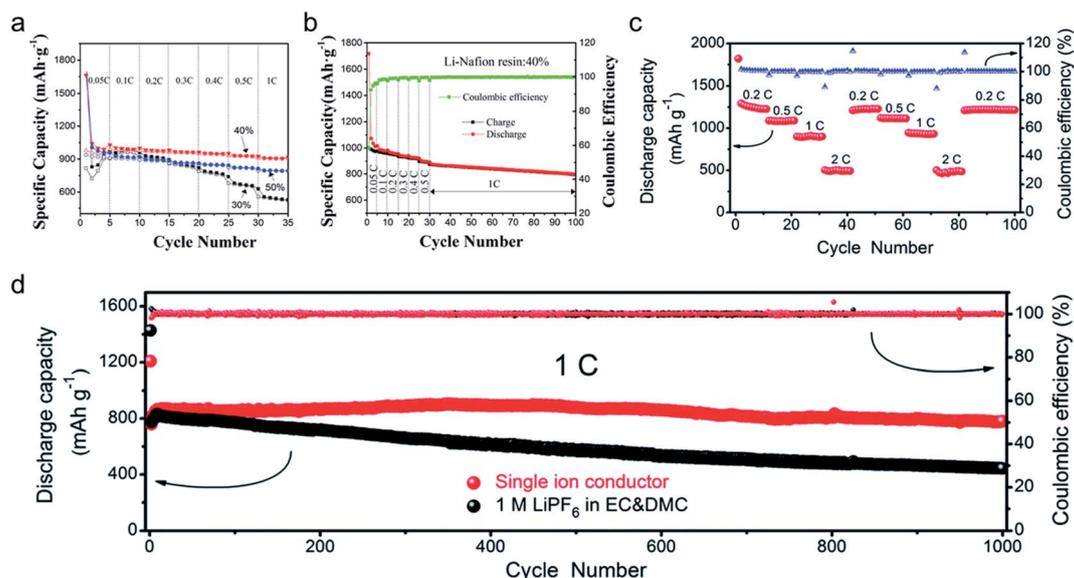
Fig. 19 Performance in Li-S batteries. The rate performance (a) and the cycling behavior (b) of the  $\text{Li}|\text{PC-Li-Nafion membrane}| \text{C-S}$  cells. (a and b) are reproduced with permission.<sup>161</sup> Copyright 2017, Elsevier. (c) Rate performance of  $\text{Li}|\text{PEMA-graft-LiATFSI}| \text{S@PAN}$  cells at various C rates and (d) cycling performances at 1C for 1000 cycles. (c and d) are reproduced with permission.<sup>162</sup> Copyright 2018, Royal Society of Chemistry.
