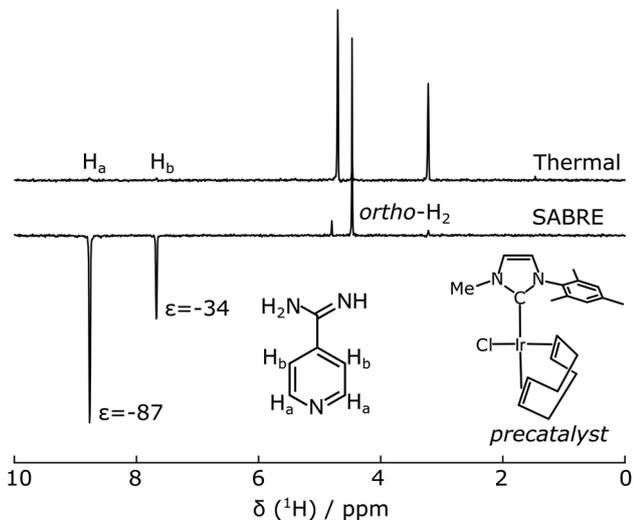
Fig. 1 400 MHz NMR spectra of 1.5 mM 4-amidinopyridine with 0.3 mM Ir(ImeMes) polarization transfer catalyst in  $d_4$ -methanol (a) non-hyperpolarized ("thermal") and (b) SABRE after bubbling for 30 s in a 6.5 mT magnetic field at 294 K, followed by acquisition at 9.4 T. The structures of the 4-amidinopyridine, and of the precatalyst before activation, are inset.
