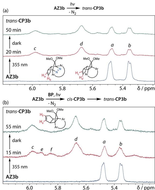
Fig. 5 *In situ*  $^1\text{H}$  NMR (400 MHz) analysis of the  $\text{N}_2$  loss of **AZ3b** in degassed toluene- $d_8$  at 199 K with Nd:YAG laser irradiation ( $\lambda_{\text{emi}} = 355$  nm, 30 mJ). (a) Direct irradiation of **AZ3b** (6.49 mM); (b) Irradiation of **AZ3b** (0.60 mM) in the presence of benzophenone (9.32 mM).
