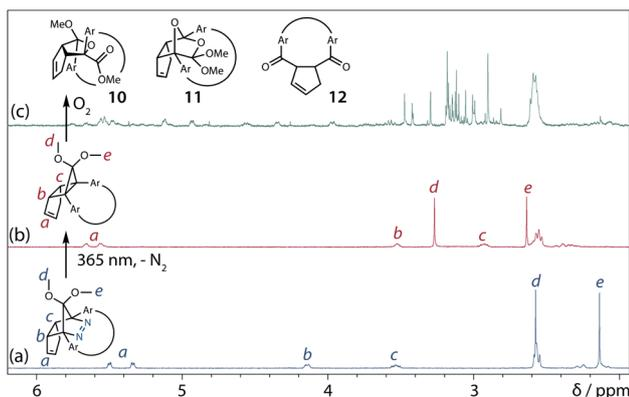
Fig. 4 *In situ*  $^1\text{H}$  NMR (400 MHz) analysis of the photoreaction of AZ3b (4.47 mM in degassed  $\text{C}_6\text{D}_6$ ).  $^1\text{H}$  NMR spectrum of (a) AZ3b before irradiation; (b) *trans*-CP3b after irradiation with a 365 nm LED lamp for 90 s at 298 K under nitrogen atmosphere; and (c) *trans*-CP3b decomposition upon exposure to air for 3 min.
