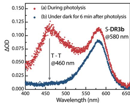
Fig. 6 Low-temperature UV-vis absorption spectra of the photolysis of **AZ3b** (2.46 mM) in a degassed MTHF matrix at 90 K.
