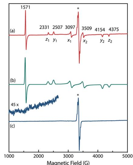
Fig. 7 Experimental EPR spectra of **AZ3b** (4.92 mM) in a MTHF matrix at 80 K (a) during photolysis and (c) in the dark after irradiation; inset: enhanced view from 1000–2670 G. (b) EPR spectrum simulated using  $D/hc = 0.096$   $\text{cm}^{-1}$  and  $E/hc = 0.019$   $\text{cm}^{-1}$ . The asterisk indicate signals that correspond to impurities in MTHF.
