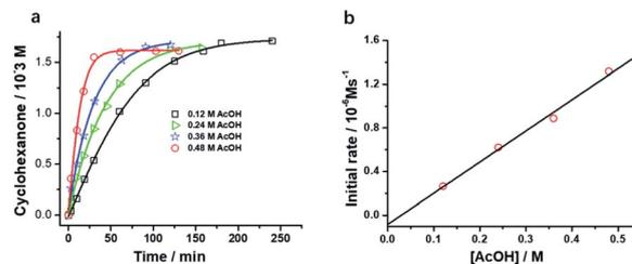
Fig. 4 (a) Effects of  $\text{CH}_3\text{CO}_2\text{H}$  on cyclohexane oxidation by  $\text{RuO}_4^-$  in  $\text{CH}_3\text{CN}$ . Conditions:  $[\text{Pr}_4\text{N}][\text{RuO}_4]$  (0.01 M), cyclohexane (1.0 M) in  $\text{CH}_3\text{CN}$  at 23 °C. (b) Plot of initial rate versus  $[\text{AcOH}]$  (slope =  $(2.72 \pm 0.13) \times 10^{-6}$ , y-intercept =  $-(3.33 \pm 3.82) \times 10^{-8}$ ,  $r = 0.9908$ ).
