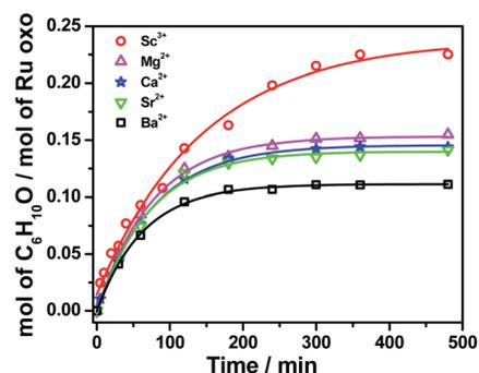
Fig. 2 Effects of various Lewis acids on cyclohexane oxidation by  $\text{RuO}_4^-$  in  $\text{CH}_3\text{CN}$ . Conditions:  $[^n\text{Pr}_4\text{N}][\text{RuO}_4^-]$  (0.01 M), Lewis acid (0.04 M), cyclohexane (1.0 M) at 23 °C.
