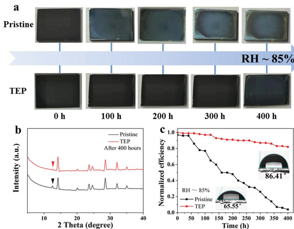
**Fig. 5** (a) Photographs of perovskite films without and with the TEP additive stored under dark conditions at  $\text{RH} \approx 85\%$  for different time periods. (b) XRD analysis of perovskite films stored under dark conditions at  $\text{RH} \approx 85\%$  for 400 hours. (c) Normalized PCE recorded under room temperature,  $\text{RH} \approx 85\%$ , dark conditions for 400 hours. The insets show the water-contact-angle of the pristine and TEP-modified perovskite films.
