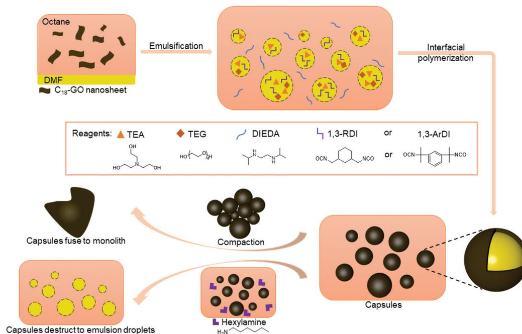
**Scheme 1** Overview of the work reported here: formation of capsules with shells containing hindered urea bonds (HUBs) and the fusion or destruction of the capsule shells. Capsules were prepared by interfacial polymerization in oil-in-oil Pickering emulsions stabilized by functionalized graphene oxide nanosheets.
