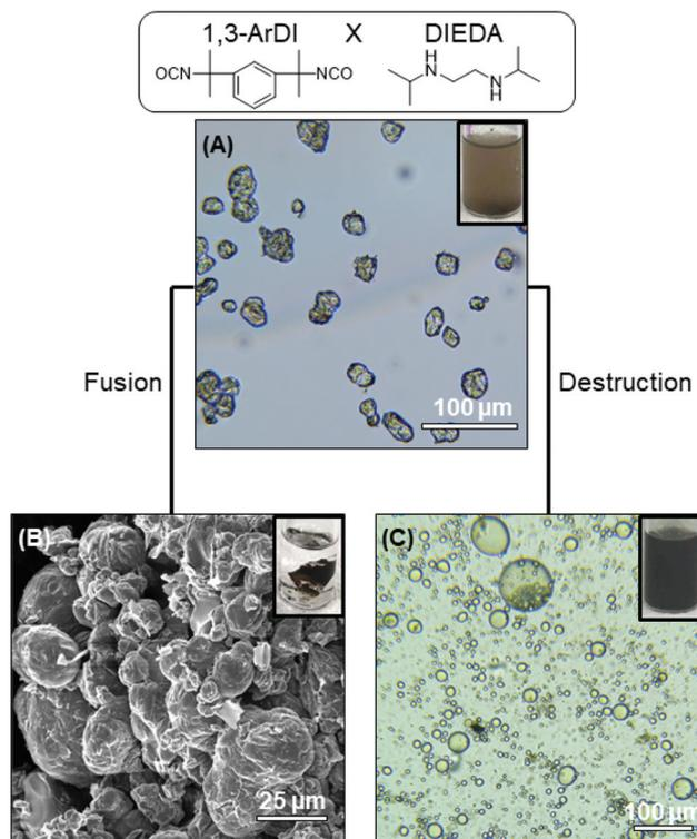
**Fig. 3** 1,3-ArDI-DIEDA capsules: (A) optical microscopy image of capsules dispersed in dodecane; (B) SEM image of monolith after capsule fusion; (C) optical microscopy image of droplets after capsule destruction by hexylamine. Inset images are photographs of the samples.
