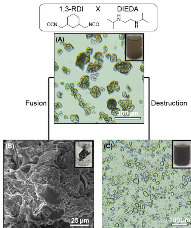
**Fig. 2** 1,3-RDI-DIEDA capsules: (A) optical microscopy image of capsules dispersed in dodecane; (B) SEM image of monolith after capsule fusion; (C) optical microscopy image of droplets after capsule destruction by hexylamine. Inset images are photographs of the samples.
