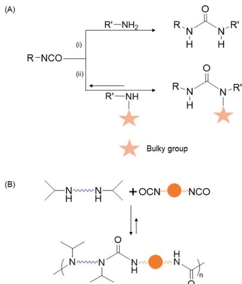
**Fig. 1** (A) Illustration of (i) irreversible urea bond formed by reaction of an isocyanate and primary amine, and (ii) reversible hindered urea bond (HUB) formed by reaction of an isocyanate and secondary amine bearing a bulky substituent; and (B) hindered polyurea chemistry.
