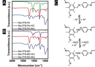
Fig. 5 FT-IR spectra (A and B) to elucidate the sensing mechanism (C).
