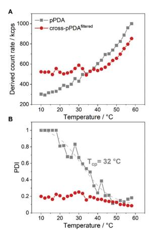
Fig. 8 Plots of the count rate (A) and PDI (B) of pPDA in 150 mM NaCl and cross-pPDA<sup>filtered</sup> at increasing temperature. The inflection point of the dashed sigmoidal fitting curve in (B) at 32 °C appears close to the cloud point of pPDA. The sample was equilibrated for 2 min at each temperature before DLS measurement.
