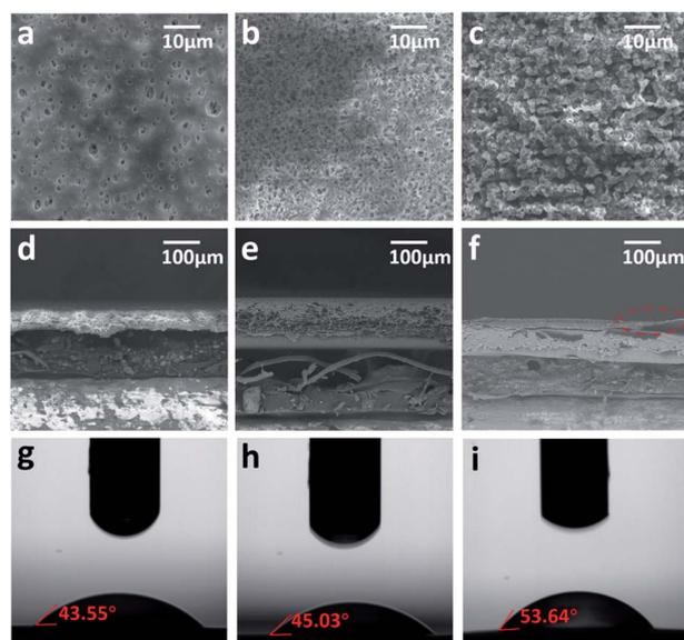
**Fig. 2** SEM images showing (a–c) top-down and (d–f) cross-sectional views of (a and d) the PES substrate, (b and e) TFC, and (c and f) HOF-TFN-2. Water-in-air contact angles for PES (g), TFC (h), and HOF-TFN-2 (i).
