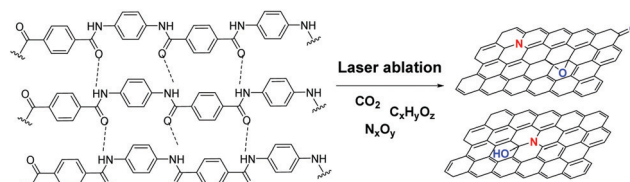
Fig. 2 Laser-induced transformation of Kevlar into graphene-functionalized material.
