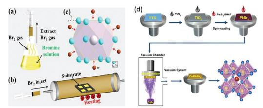
Fig. 8 (a)  $Br_2$  vapor extraction from a bottle of Br water; (b) schematics of the  $Br_2$  vapor-assisted CVD process; and (c) crystal structure. Reproduced with permission ref. 121. Copyright 2018, Elsevier Ltd. (d) Illustration of the evaporation-assisted solution method (EAS) to prepare a CsPbBr<sub>3</sub> thin film. Reproduced with permission ref. 120. Copyright 2019, American Chemical Society.
