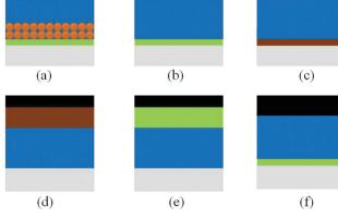
Fig. 13 Main types of device structure of PSCs. (a) Regular mesoscopic structure. (b) Regular planar structure. (c) Inverted (planar) structure. (d) ETL-free structure. (e and f) HTL-free structure.
