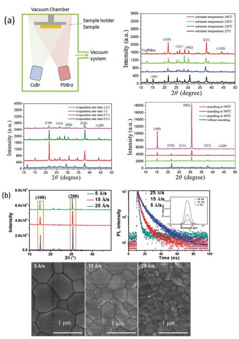
Fig. 10 (a) Representation of the vacuum dual-source thermal co-evaporation process for the preparation of CsPbBr<sub>3</sub> films. Reproduced with permission ref. 124. Copyright 2020, Elsevier Ltd. (b) Corresponding SEM micrographs of the CsPbBr3 films evaporated at different rates. Reproduced with permission ref. 125. Copyright 2018, Wiley-VCH.
