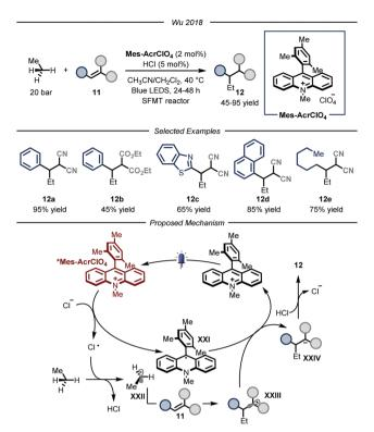
Fig. 8 Use of chlorine radical as HAT catalyst for the activation of ethane. LED: light emitting diode; SFMT: stopped flow microreactor.
