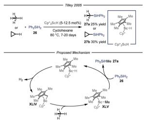
Fig. 16 Scandium-catalyzed silylation of light alkanes through C-H activation. Cp\*: pentamethylyclopentadienyl
