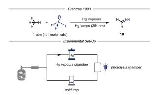
Fig. 12 Functionalization of methane using ammonia and Hg
