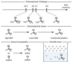
Fig. 1 General representation of the issues related to functionalization of gaseous alkanes. BDE: bond dissociation energy; FG:
