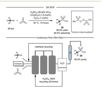
Fig. 18 Highly selective conversion of methane and sulfur trioxide into methanesulfonic acid
