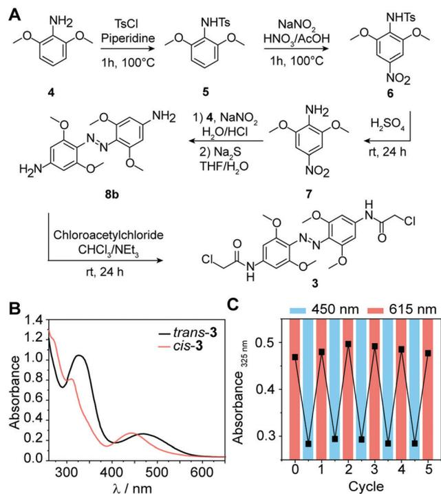
**Fig. 2** (A) Synthesis scheme of tetra-*ortho*-methoxy substituted azobenzene. (B) Absorbance spectra of 1 mM **3** in DMSO before and after irradiation with  $\lambda = 615$  nm for 30 min. (C) Repeated irradiation cycles of **3** using 615 nm for *trans*-to-*cis* and 450 nm for *cis*-to-*trans* isomerization.
