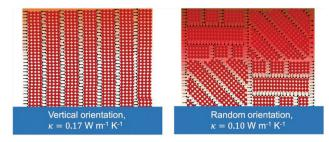
Fig. 12 Schematic illustrations of vertically and randomly oriented BA2MA3Pb4l13 crystal orientations that lead to different thermal conductivities. Reprinted with permission from ref. 32. Copyright (2020) American Chemical Society
