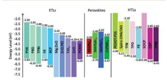
**Fig. 11** Energy level alignment of various materials used as ETLs and HTLs in perovskite devices. From ref. 192. Reprinted with permission from Flsevier
