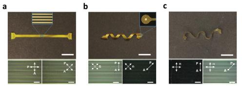
Fig. 4 Photo images of 16-channel multielectrode arrays fabricated on LCE substrates in various 2D and 3D shapes. (a) 'Flat'. Inset shows multichannel gold traces. (Scale bar = 1 cm.) (b) 'Twisted'. Inset shows exposed site of gold microelectrode. (Scale bar = 1 cm.) (c) 'Wavy'. (Scale bar = 1 cm.) The bottom images are polarized optical micrographs of each device. (Scale bars = 500  $\mu$ m.)
