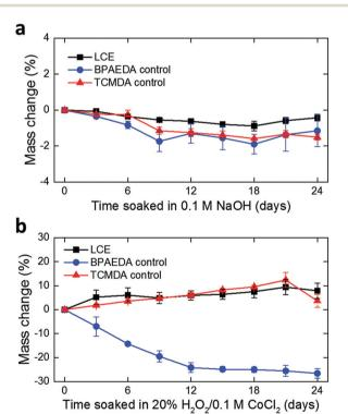
Fig. 2 Monitoring of mass change in LCE and control films over 24 days in (a) 0.1 M NaOH (mean  $\pm$  SD, n = 4) and (b) 20% H<sub>2</sub>O<sub>2</sub>/0.1 M CoCl<sub>2</sub> (mean  $\pm$  SD, n = 4), both at 37 °C.
