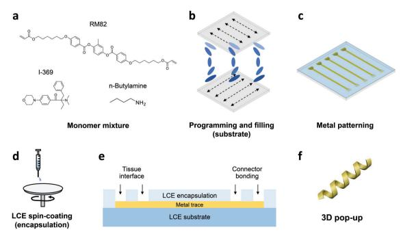
Fig. 1 Schematic illustration of fabrication procedure of LCE-based 3D, implantable electronics. (a) Monomer mixture. (b) Programming and filling (c) Metal patterning. (d) LCE spin-coating. (e) Selective metal exposure. (f) 3D pop-up
