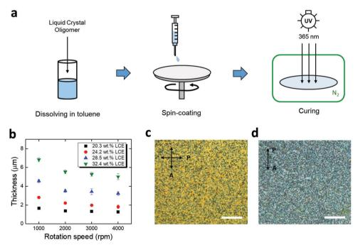
Fig. 3 (a) Schematic illustration of LCE spin-coating process. (b) Thickness of spin-coated LCE films as functions of LCE concentration and rotation speed (mean  $\pm$  SD, n = 3). Polarized optical micrographs of spin-coated LCE (c) on a gold trace (viewed in reflection mode) and (d) on a twisted nematic LCE substrate (viewed in transmission mode). (Scale bars =  $30 \mu m$ .)
