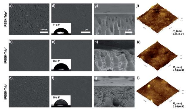
Fig. 3 Typical iPEEK membrane surface morphology at high (a-c) and low (d-f) magnifications, and cross-sectional images (g-i). The inset images are water contact angles (WCAs) of the membrane surface. Surface roughness shown by AFM images (j-l).
