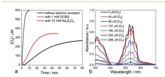
Fig. 4 (a) Time courses of oxygen evolution from water measured by a platinum Clark electrode in the absence of an electron acceptor (black) and in the presence of DCBQ (red) and  ${\rm S_2O_8}^{2-}$  as electron acceptors (blue). (b) Titration of  ${\rm H_2O_2}$  with KMnO<sub>4</sub> at different concentrations of photoproduced O<sub>2</sub> in the absence of an electron acceptor.
