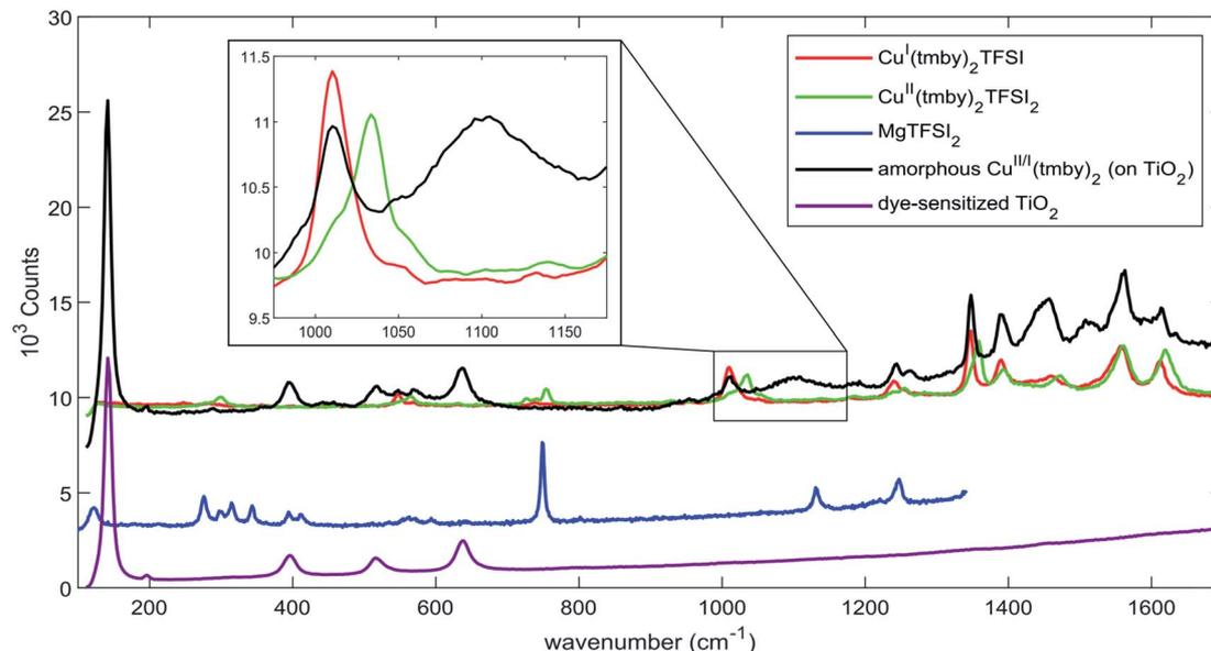
Fig. 4 Raman spectra of  $\text{Cu}^{\text{II}}(\text{tmby})_2 \text{TFSI}_{(2)}$  and  $\text{MgTFSI}_2$  (powders), DSCs sensitized with the XY1:L1 sensitizer combination as well as (sensitized) DSCs containing amorphous  $\text{Cu}^{\text{III}}(\text{tmby})_2 \text{TFSI}_{(2)}$  hole transport material. The two latter spectra were recorded inside the 'sandwich' DSC. Spectra are offset for clarity.
