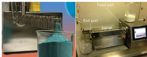
Fig. 23 Twin-screw extruder with key parts highlighted. The two screws which convey and knead the reactants are housed in the barrel.
