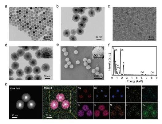
Fig. 1 Structural and compositional characterization of UMNOCC-PEG nanoparticles. TEM images of (a) the NaGdF<sub>4</sub>:Yb,Er core nanoparticles, (b) UCNP@dMSN-SNO, (c) CuO<sub>2</sub> nanodots, and (d) UMNOCC-PEG nanoparticles. (e) SEM image and (f) corresponding EDS spectrum of the UMNOCC-PEG nanoparticles. (g) Dark-field STEM image and the corresponding elemental mappings of UMNOCC-PEG nanoparticles.
