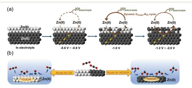
Fig. 7 (a) Schematic process of the zinc electrocatalyst during the CO<sub>2</sub>RR. (b) Schematic mechanisms of the CO<sub>2</sub>RR for Zn(II) and Zn(0) electrocatalysts.
