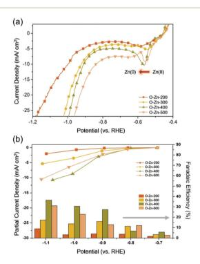
Fig. 3 CO<sub>2</sub>RR performance analysis (a) LSV measurements of O-Zn-200, O-Zn-300, O-Zn-400 and O-Zn-500. Partial current density (up in b) and faradaic efficiency (bottom in b) of formate of O-Zn-200, O-Zn-300, O-Zn-400 and O-Zn-500 in a selected potential window of 0.70 to -1.10 V (vs. RHE).
