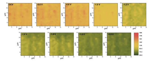
Fig. 5 In situ Raman mapping of O-Zn-400 (15  $\times$  15  $\mu$ m<sup>2</sup>) based on the peak intensity at 566 cm<sup>-1</sup>.
