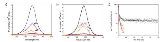
Fig. 7 Steady-state photoluminescence spectra of FTO/TiO<sub>2</sub>/perovskite (black), FTO/TiO<sub>2</sub>/perovskite/Spiro-MeOTAD (purple) and FTO/TiO<sub>2</sub>/perovskite/D35/Spiro-MeOTAD (orange) devices at room temperature upon excitation at (a) 482 nm and (b) 650 nm. (c) Time-correlated single photon counting spectra under 482 nm excitation probed at 750 nm obtained at room temperature.
