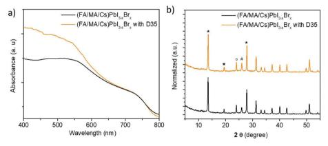
Fig. 2 UV-vis absorption spectra (a) and XRPD patterns (b) of mixed perovskite films with and without D35 treatment. Symbols "\*", "o" and "#" represent the perovskite, FTO and TiO<sub>2</sub> peaks, respectively.
