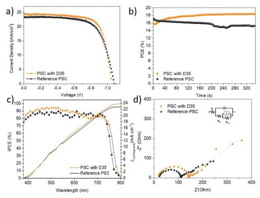
Fig. 6 The J-V curves of the best performing cells with and without D35 (a); the steady-state power conversion efficiency outputs under 1 sun illumination for reference and modified PSCs (b); the IPCE spectra and integration currents of the corresponding PSCs (c); the Nyquist plots obtained via EIS measurements, under 1 sun illumination and under  $V_{MPP}$  bias. Fitting of data is performed using the equivalent electrical circuit in the inset
