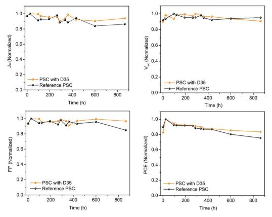
Fig. 9 Evolution of the main photovoltaic parameters over time for PSCs with and without D35.
