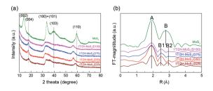
Fig. 1 (a) XRD patterns, (b) FT-EXAFS spectra of 1T/2H-MoS<sub>2</sub> (D25), 1T/ 2H-MoS<sub>2</sub> (D50), 1T/2H-MoS<sub>2</sub> (D75), 1T/2H-MoS<sub>2</sub> (D100) and MoS<sub>2</sub>.
