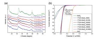
Fig. 6 (a) XRD patterns of 1T/2H-MoS<sub>2</sub> (N50), 1T/2H-MoS<sub>2</sub> (N100), 1T/ 2H-MoS<sub>2</sub> (N200), 1T/2H-MoS<sub>2</sub> (N400), 1T/2H-MoS<sub>2</sub> (N800), 1T/2H-MoS<sub>2</sub> (N1600) and MoS2. (b) Linear sweep voltammetry (LSV) curves of 1T/ 2H-MoS<sub>2</sub> (N50), 1T/2H-MoS<sub>2</sub> (N100), 1T/2H-MoS<sub>2</sub> (N200), 1T/2H-MoS<sub>2</sub> (N400), 1T/2H-MoS<sub>2</sub> (N800), 1T/2H-MoS<sub>2</sub> (N1600) MoS<sub>2</sub>, and Pt/C.
