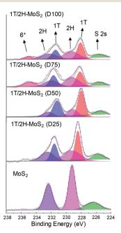
Fig. 2 Mo 3d XPS spectra of 1T/2H-MoS<sub>2</sub> (D25), 1T/2H-MoS<sub>2</sub> (D50), 1T/ 2H-MoS<sub>2</sub> (D75), 1T/2H-MoS<sub>2</sub> (D100) and MoS<sub>2</sub>.
