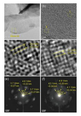
**Fig. 3** (a), (b) High-resolution TEM bright field images of 1T/2H-MoS<sub>2</sub>, (c), (d) zoom in of area 1 and 2 respectively, and (e), (f) selected area electron diffraction (SAED) of area 1 and 2, respectively.
