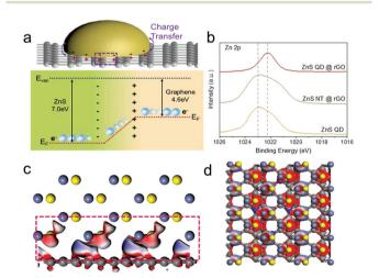
Fig. 4 (a) Schematic demonstration of the electron distribution at the interface between graphene and ZnS. (b) Zn 2p peaks of the XPS pattern of ZnS QD@rGO, ZnS NT@rGO, and pure ZnS QDs. (c and d) The charge distribution calculated by density functional theory at the interface of ZnS QDs and N-rGO from the top (c) and side views (d).
