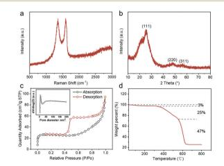
Fig. 2 Raman pattern (a), XRD pattern (b), BET surface area (c) (pore size distribution inset), and TGA curve of the as-synthesized ZnS QD@rGO (d).
