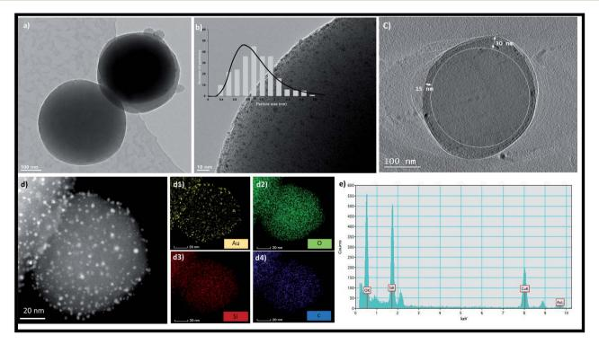
Fig. 1 (a and b) Bright-field TEM image, (c) volume-slice electron tomography image. (d) HAADF-STEM image, and STEM EDX mappings of AuNCs/MSN-NH<sub>2</sub>: Au, O, Si, and O are shown in (d1-d4), respectively. (e) EDX spectrum of AuNCs/MSN-NH<sub>2</sub>.
