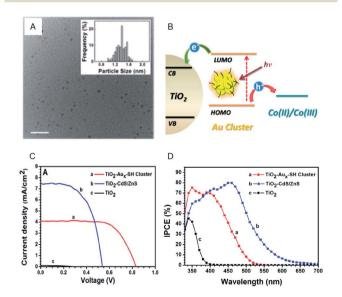
Fig. 13 (A) TEM image of Au<sub>x</sub>-SG cluster. Scale bar shows the length of 10 nm. (B) Schematic of the working principle of metal-NC-sensitized solar cells. (C) J-V characteristics. (D) IPCE spectra of TiO<sub>2</sub> modified with Au<sub>x</sub>-SH cluster, TiO<sub>2</sub> modified with CdS/ZnS and TiO<sub>2</sub> electrodes. Panels (a) – (d) are reproduced with permission from ref. 75. Copyright 2013 American Chemical Society.
