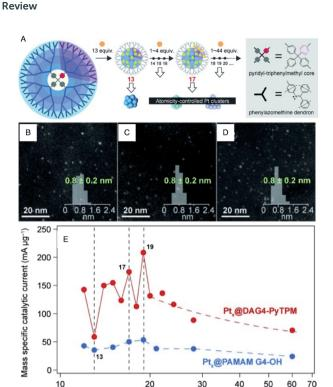
Fig. 7 (A) Illustration of the precise synthesis method of atomicity precise Pt NCs using a dendrimer reactor. HAADF-STEM images of (B)  $Pt_{13}$ , (C)  $Pt_{17}$  and (D)  $Pt_{19}$  NCs. (E) Variations of the mass ORR activity vs. the atomicity of the Pt NCs. Panels (a)-(e) are reproduced with permission from ref. 45. Copyright 2015 Wiley-VCH.
