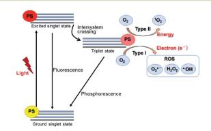
**Fig. 15** Schematic Jablonski's diagram of Type I and Type II reactions in PDT. PS: photosensitizer.
