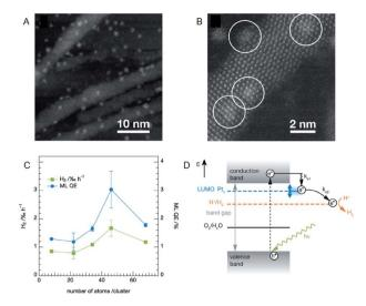
Fig. 9 (A) and (B) HAADF-STEM images of CdS nanorods decorated with Pt NCs at different magnification. (C) Photocatalytic activity of the CdS nanorods decorated with size-selected Pt NCs as a function of cluster size. (D) Reaction pathways for the photocatalytic H<sub>2</sub> evolution in CdS with Pt NCs. Panels (a)–(d) are reproduced with permission from ref. 58. Copyright 2013 American Chemical Society.
