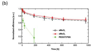
Fig. 8 (a) X-Ray photoelectron spectroscopy of solution-processed MoO<sub>τ</sub> (sMoO<sub>τ</sub>) compared to an evaporated film (eMoO<sub>τ</sub>) and (b) stability of OPV devices with P3HT:PC<sub>61</sub>BM active layer, stored in ambient conditions reported by Rand et al.<sup>60</sup> Reprinted with permission from ref. 60. Copyright 2011 American Chemical Society
