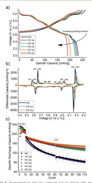
Fig. 5 Electrochemical data for undoped and Ga-doped LNO from galvanostatic cycling of half-cells at 25  $^{\circ}$ C in the voltage range between 3.0 and 4.3 V vs. Li<sup>+</sup>/Li. (a) 1st cycle voltage profiles. (b) 3rd cycle differential capacity plots. Only selected samples are shown for clarity. (c) Specific discharge capacity over 110 cycles.
