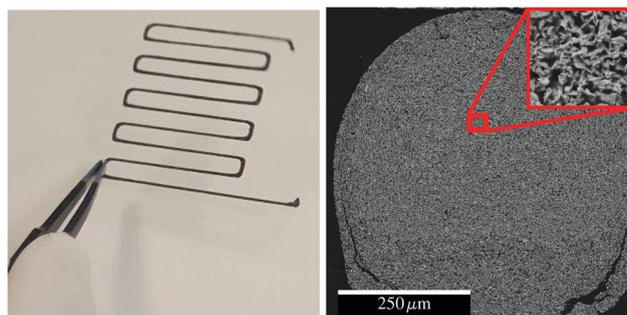
**Fig. 2** (a) Free-standing printed conductive structure after reaction of printed ball milled powders. (b) Cross-sectional electron micrograph of reacted conductive line, demonstrating bi-continuous microstructure.
