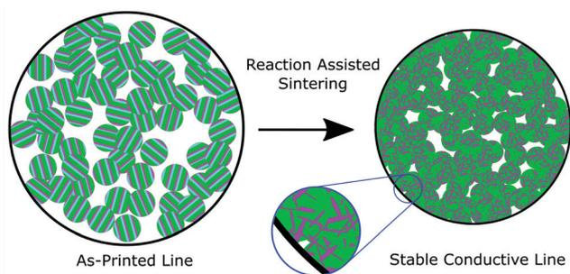
**Fig. 1** Schematic cross section of a 3D printed RAIL filament – A/B/C tri-layered particles on the left undergo a reaction to form a new AB phase in a matrix of C, resulting in a small volume shrinkage.
