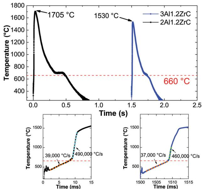
**Fig. 4** (top) Temperature vs. time data from pyrometry on 2Al and 3Al thin films ignited by electric spark. (bottom) Expanded data at the start of reaction, demonstrating a rapid increase in heating rate after passing the Al melting temperature. Horizontal offset of 1.5 s applied to the 3Al data for clarity.
