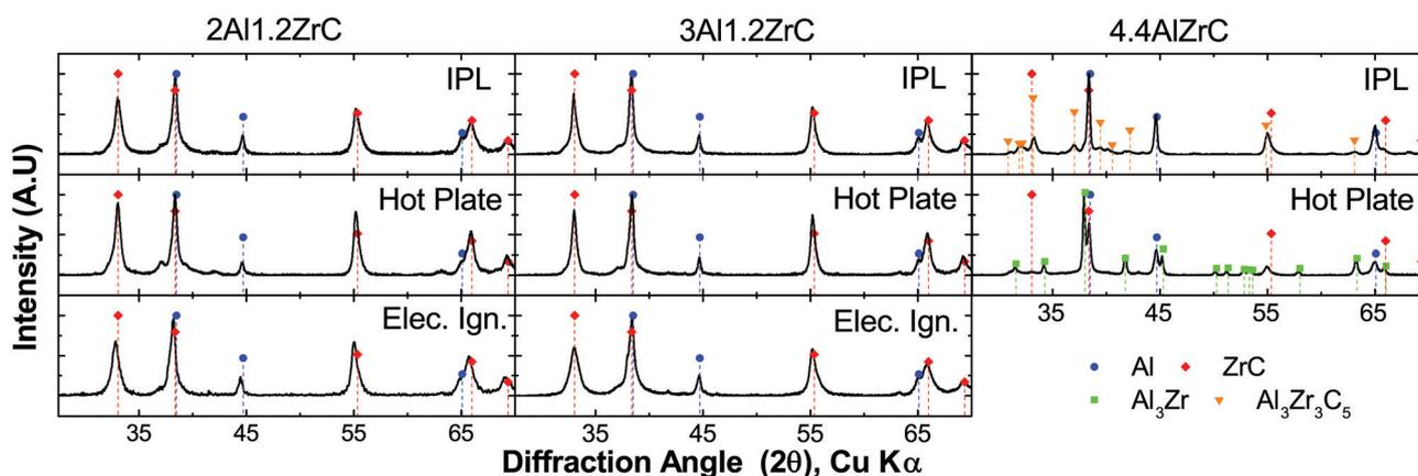
**Fig. 3** Comparison of phases formed in 2Al, 3Al and 4.4Al thin films after reactions ignited by IPL, hot plate, and electric spark. Arranged in order of decreasing uniformity of energy delivery to the sample during ignition, demonstrating that for compositions too rich in Al, only very uniform ignition can produce the desired product phases. Note that 4.4Al foils would not propagate from an electric spark.
