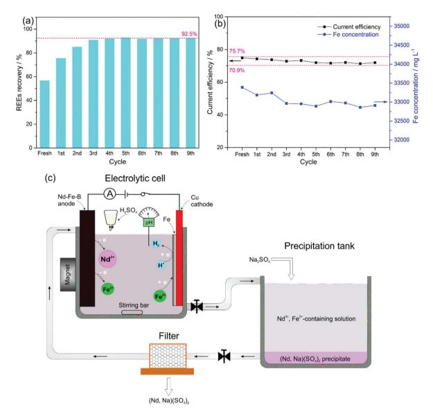
Fig. 4 (a) Percentage extraction of REEs at an anodic current density of 25 mA cm $^{-2}$  and a cathodic current density of 12.5 mA cm $^{-2}$  and (b) current efficiency of Fe deposition and total dissolved Fe concentration over 9 recycling cycles. (c) Schematic of the proposed closed-loop recycling route for recovering REEs from the sintered Nd-Fe-B magnets.
