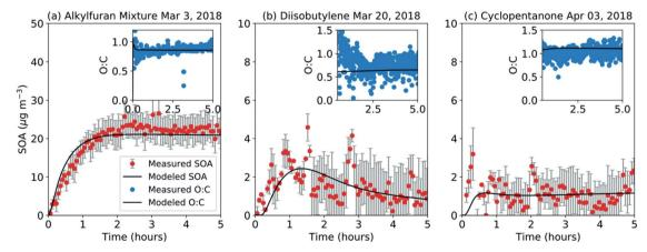
Fig. 2 SOM-TOMAS model predictions based on parameter fits (solid black lines) compared to measurements (symbols) of SOA mass concentrations and SOA O: C for the (a) alkylfuran mixture, (b) diisobutylene, and (c) cyclopentanone. Model predictions for O: C are shown only after the first half hour as they were found to be unreliable at earlier times when the SOA mass concentrations were lower than 0.5  $\mu$ g m<sup>-3</sup>.
