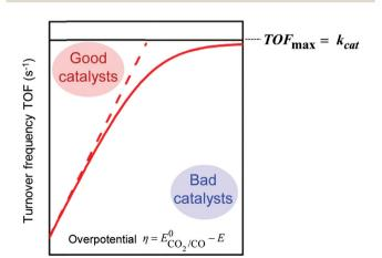
Fig. 1 Benchmarking of molecular catalyst intrinsic properties for the  $CO_2$ -to-CO reduction through the catalytic Tafel plot [TOF =  $f(\eta)$ ].
