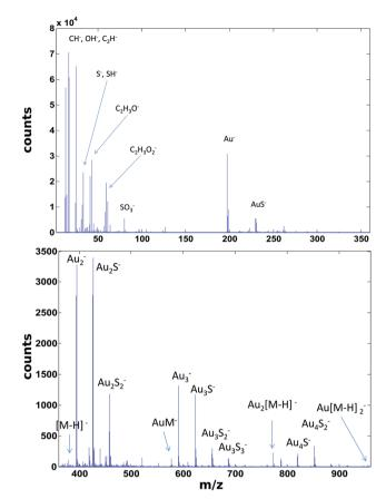
Fig. 4 ToF-SIMS negative ion spectrum from the PEG4thiol SAM.
