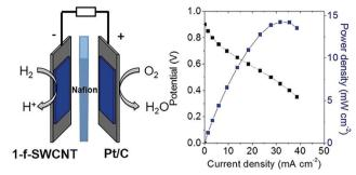
**Fig. 11** Polarization (black) and power density (blue) curves for an MEA employing  $[Ni(P_2^{Cy}N_2^{Arg})_2]^{7+}$  (denoted as 1-f-SWCNT) and Pt/C as the anode and cathode catalysts, respectively. Experimental conditions: anode loading: 0.3  $\mu$ g cm<sup>-2</sup>, cathode loading (Pt/C): 1 mg cm<sup>-2</sup>, Nafion<sup>®</sup> as the polymer electrolyte, 60 °C cell temperature. Reprinted with permission from ref. 297. Copyright 2017 Wiley-VCH.
