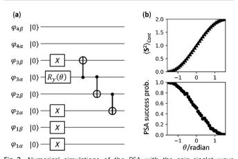
Fig. 2 Numerical simulations of the PSA with the spin-singlet wave function contaminated by spin-triplet states. (a) A quantum circuit for the preparation of  $|\Psi_{\text{Cont}}\rangle$  given in eqn (11). (b) The  $\langle \mathbf{S}^2\rangle$  value of the spin contaminated wave function  $|\Psi_{\text{Cont}}\rangle$  (Top) and the PSA success probability calculated from the numerical quantum circuit simulations (Bottom).
