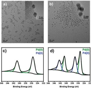
Fig. 1 (a and b) TEM images and (c and d) XPS spectra at the Pd 3d level of (a and c) the pristine and (b and d) oxidized Pd NPs after the treatment with  $[Ph_2!]BF_4$ .
