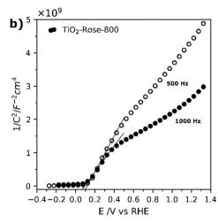
Fig. 10 (a) Nyquist plots of  $TiO_2$ -Rose-800 at the open circuit potential (OCP) of the cell under 1 sun illumination (AM 1.5G, 100 mW cm<sup>-2</sup>). (b) Mott–Schottky plots at a fixed frequency of 500 Hz and 1000 Hz of  $TiO_2$ -Rose-800 in 1 M KOH (pH = 13.6).
