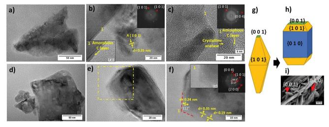
Fig. 4 TEM and HRTEM micrographs of (a-c) TiO<sub>2</sub>-Rose-AD and (d-f) TiO<sub>2</sub>-Rose-800. Fast Fourier transformation (FFT) patterns and inverse FFT image are shown in the inset of (b and c) and (f). (f) Region highlighted in (e). (g) Wulff construction of anatase crystals and (h) evolved shape with high exposure of {0 1 0} facets. (i) SEM micrograph highlighting the facets.
