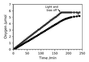
Fig. 11 Amount of  $O_2$  gas evolved at 1.23  $V_{RHE}$  under simulated sunlight (AM 1.5G, 100 mW cm $^{-2}$ ). The amount of  $O_2$  quantified with a fluorescence probe is represented by solid markers, whereas the theoretical amount of  $O_2$  calculated assuming a 100% faradaic efficiency is shown with empty markers.
