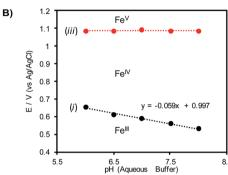
Fig. 2 (A) Differential pulse voltammograms of 0.5 mM 1 in 1:1  $\rm CH_3CN$ : buffer (0.1 M phosphate). (B) Pourbaix diagram derived from the peak potentials of redox features (i) and (iii) in (A).
