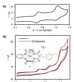
Fig. 1 (A) CV of [(TAML)Fe $^{III}$ (OH $_2$ )]Na (1) in CH $_3$ CN (0.1 M LiClO $_4$ ). (B) CVs of 0.5 mM 1 in the absence (black) and presence (red) of 20 mM ethylbenzene in 1 : 1 CH $_3$ CN : H $_2$ O and K $_2$ HPO $_4$  (0.1 M). The increase in the current of the (TAML)Fe redox feature at 1.25 V (vs. Ag/AgCl) is attributed to catalytic ethylbenzene oxidation by a high-valent Fe-oxo species generated at this potential. Scan rate = 50 mV s $^{-1}$ .
