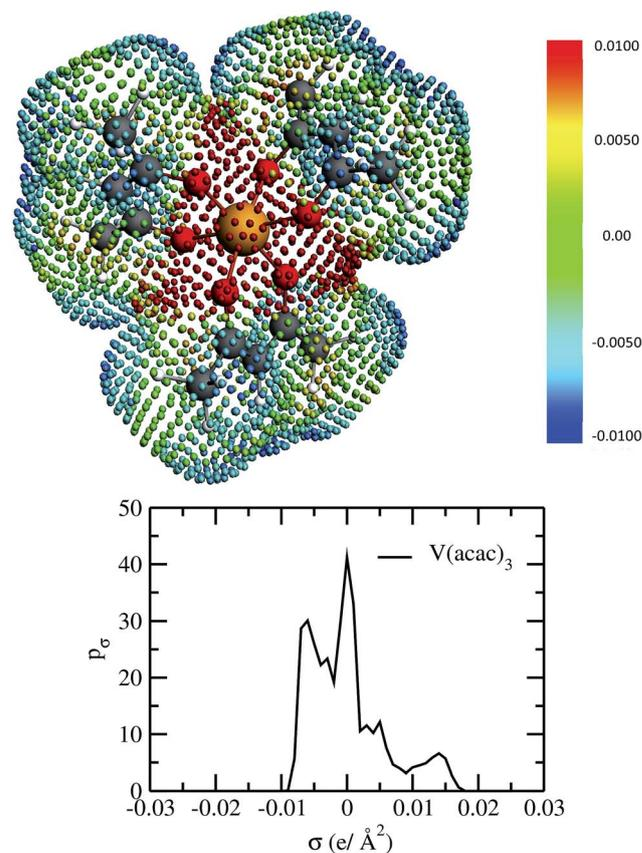
Fig. 2 The COSMO surface charge points of V(acac)<sub>3</sub> has been shown above with the color bar representing the COSMO charge density. The corresponding  $\sigma$  profile of V(acac)<sub>3</sub> has been shown below.
