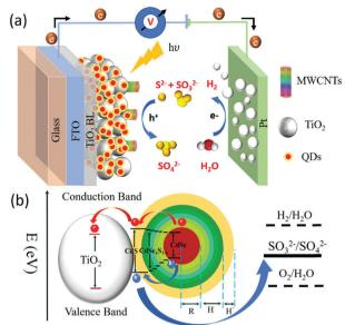
Fig. 1 Schematic illustration of the: (a) PEC device working principle for H<sub>2</sub> generation; (b) band structure of the graded alloyed core/shell QDs (R = radius of CdSe core; H = thickness of the graded alloyed interfacial)layers; H' = thickness of the outer CdS layer) sensitized TiO<sub>2</sub>-MWCNT hybrid film applied as the working electrode. The arrows show the electron and hole transfer process.
