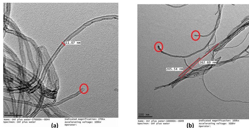
Fig. 9 TEM micrographs of FMWCNTs showing (a) a diameter of 10–20 nm (marked in red circles) and (b) a length of 0.1–1 \mu\text{m} .
