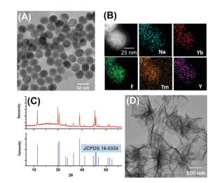
Fig. 1 TEM (A), EDS mapping (B) and X-ray diffraction (XRD) patterns (C) of NaYF<sub>4</sub>:Yb,Tm UCNPs; (D) TEM of MnO<sub>2</sub> nanosheets.
