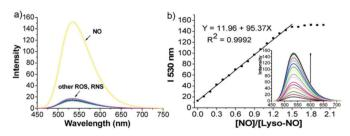
Fig. 102 (a) Selectivity of 63 (11 µM) fluorescence response for NO over other reactive nitrogen and oxygen species (5.0 equiv.) in 20:80 CH<sub>3</sub>CN-H<sub>2</sub>O solution at pH 5.0 (in 10 mM phosphate buffer). (b) Intensity at 530 nm vs. NO concentration under the same conditions. Inset: Changes in fluorescence spectra of 63 (11 µM) upon addition of different amounts NO solution (0-2.0 equiv.). Copyright 2012 American Chemical Society.
