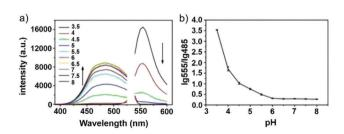
Fig. 19 pH dependent ratiometric fluorescence emission of probe 15. (a) Fluorescence emission spectra of probe 15 (10  $\mu g$  mL<sup>-1</sup>) at pH 3.5-8.0 under dual-wavelength excitation ( $\lambda_{ex}$ @300 nm for dansyl group, 532 nm for R6G-lactam). (b) pH titration curves of lg ratios between fluorescence emission of R6G-amide (I<sub>555nm</sub>) and that of dansyl group (I<sub>485nm</sub>). Copyright 2013 Elsevier.
