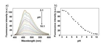
Fig. 34 (a) The fluorescence change of probe 23 in Britton-Robinson buffer at different pH values; (b) the fluorescence intensity at 460 nm depending on different pH values,  $\lambda_{ex}$  = 360 nm. Copyright 2013 Royal Society of Chemistry.
