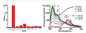
Fig. 82 (a) Fluorescence ratio (512/586) change of probe **54** towards different ROS. (b) Changes of fluorescence wavelength of probe **54** in pH  $\sim 5$  PBS (containing 30% methanol) in the presence of 1  $\mu M$  hemin and 1 mM CumOOH, excited at 488 nm. Copyright 2015 American Chemical Society.
