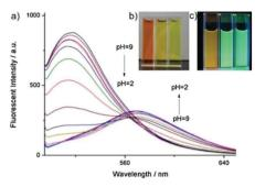
Fig. 50 (a) Fluorescence spectra ( $\lambda_{ex}$  = 480 nm) of probe 35 (2  $\mu$ M) at different pH values; (b) the color change of probe 35 (1 mM) in 20 mM PBS buffer at different pH values under the condition of visible light; (c) the color change of probe 35 (1 mM) in 20 mM PBS buffer at different pH values under UV light irradiation. Copyright 2014 Elsevier.
