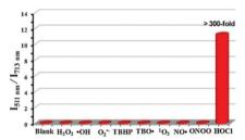
Fig. 75 Fluorescence responses ( $I_{511nm}/I_{713nm}$ ) of probe **51** (5  $\mu$ M) toward HOCl (10  $\mu$ M) and other ROS (100  $\mu$ M) in PBS (10 mM) solution (ethanol/ water = 1/1, v/v, pH 7.4);  $\lambda_{ex}$ = 480 nm, 635 nm. Copyright 2017 Elsevier.
