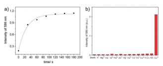
Fig. 114 (a) Fluorescence intensities at 586 nm of 68 (10 μm) in the presence of Cu<sup>2+</sup> (30 equiv.) for continuous monitoring at time interval periods (0–180 s) in PBS buffer, pH 4.7, containing 50% CH<sub>3</sub>CN as a cosolvent. Excitation at 360 nm. (b) Fluorescence intensity of the probe 68 (10 mM) at 580 nm in the presence of various analytes (30 equiv.) in PBS buffer (pH 4.7, containing 50% CH<sub>3</sub>CN as a cosolvent). Copyright 2015 Royal Society of Chemistry.
