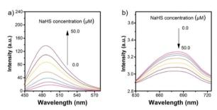
**Fig. 93** The changes of fluorescence spectra of **58** in the presence of different concentrations (0.0, 5.0, 10.0, 17.0, 20.0, 40.0, and 50.0  $\mu$ M) of NaHS in FBS. (a)  $\lambda_{\rm ex}=435$  nm; (b)  $\lambda_{\rm ex}=510$  nm. Copyright 2017 Royal Society of Chemistry.
