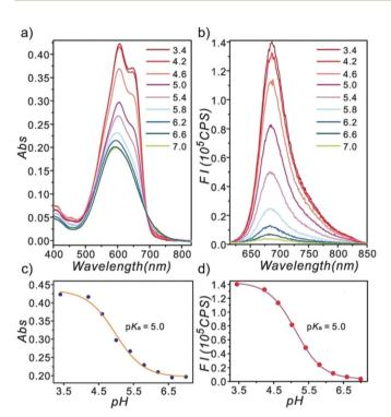
Fig. 38 Optical responses of probe **26a** towards various pH values with disodium hydrogen phosphate–citric acid buffers containing 1% DMSO. (a) Absorption spectra; (b) emission spectra ( $\lambda_{\rm ex}$  = 600 nm); (c) absorption changes with different pH values monitored at 607 nm; (d) fluorescence intensity changes with different pH values monitored at 686 nm. Copyright 2013 Royal Society of Chemistry.
