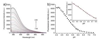
Fig. 57 (a) Fluorescence spectra of probe 38 (1 μM) in buffers at different pH values; (b) fluorescence intensity at 583 nm with pH values according to the fluorescence pH titration (pH 4.00–7.40),  $\lambda_{ex}$  = 563 nm. The inset shows the linear relationship of fluorescence intensity at 583 nm and pH values from 4.20 to 6.00 (R = 0.99523). Copyright 2015 Royal Society of Chemistry.
