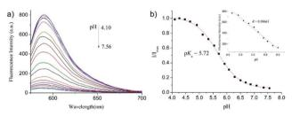
Fig. 7 (a) Fluorescence spectra of probe 4 (10  $\mu M$ ) in aqueous solution (Britton-Robinson buffer-EtOH, 9:1, v/v) with different pH values; (b) pH titration curve of probe **4**,  $\lambda_{\rm ex}$  = 563 nm,  $\lambda_{\rm em}$  = 589 nm. The inset shows the linear relationship of fluorescence intensity at 589 nm and varying pH values from 4.6 to 6.5. Copyright 2014 Elsevier.
