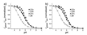
Fig. 41 (a) Plots of  $I_{green}/I_{iso}$  versus pH for probes 27a-c and 28 determined in one-photon mode. The excitation wavelength is 360 nm. (b) Plots of Igreen/  $I_{iso}$  versus pH for probe **27a-c** and **28** determined in two photon mode. Data in (b) are normalized at the maximum  $I_{\text{green}}/I_{\text{iso}}$ . The excitation wavelength for two-photon mode is 740 nm. Copyright 2013 American Chemical Society.
