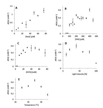
Fig. 1 Influence of some reaction parameters on the rate of the photoenzymatic epoxidation of styrene. General conditions (unless indicated otherwise in the figure): [styrene] $_0$  = 5 mM, [StyA] = 20  $\mu$ M, [FAD] = 200  $\mu$ M, [EDTA] = 20 mM, catalase = 600 U ml $^{-1}$ , [DMSO] = 1.25% (v/v), 100 mM KPi buffer (pH 7), 30 °C, stirring at 300 rpm, light intensity of 20% for 1 h. Error bars show the standard deviation for three independent experiments.
