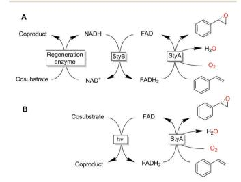
Scheme 1 Comparison of the traditional regeneration system for StyA involving two additional enzymes (A) and the nicotinamide cofactor with the simplified, direct photochemical regeneration of  $FADH_2$  (B).
