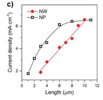
Fig. 4 Performance of the rutile TiO<sub>2</sub> NW and NP-based solar cells. (a) Dependence of the electron collection efficiency on the NW length and NP-film thickness. (b) Comparison of the current density-voltage characteristics of the NW-based cells under AM 1.5 illumination. (c) Dependence of current density on the NW length and NP-film thickness
