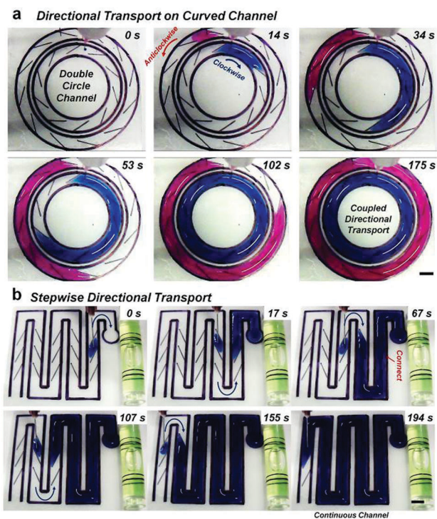
Fig. 5 Directional transport experiments on channels with complex shapes. (a) Unidirectional liquid delivery on a double circular channel. Anticlockwise and clockwise liquid transporting processes can be achieved simultaneously on the same surface by incorporating barrier spines with different directions. (b) Stepwise and programmed unidirectional liquid transport on a polygonal channel. No matter where the droplets are discharged, liquid always spreads against the direction of the spine tilt. Moreover, the asymmetric water barriers allow liquid mixing, connection, and transport from the rear to the front of the channel. Scale bar is 5 mm.
